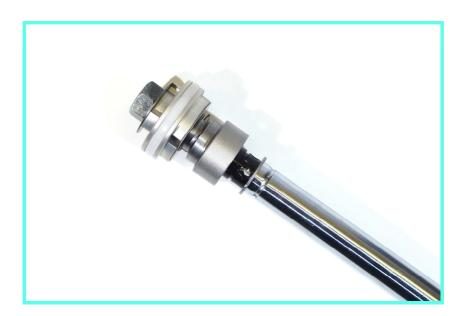
The primal damping works linear and oil flows only through one regulated orifice (hole). Too little damping and your fork comes up too fast and produces haphazard and uncomfortable ride over even the smallest rocks and bumps.
